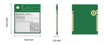
FC41D is a cutting-edge MCU Wi-Fi and Bluetooth module launched by Quectel. It boasts a high-performance processor with a frequency of up to 120 MHz and supports IEEE 802.11b/g/n protocol and Bluetooth 5.2. The module features built-in 256 KB RAM and 2 MB/4 MB flash, ensuring efficient performance. In addition, it complies with WPA-PSK, WPA2-PSK and WPA3-SAE security standards.
